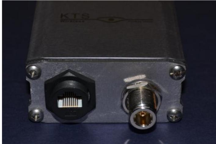
External Interfaces –Ethernet (PoE) and Antenna Port
